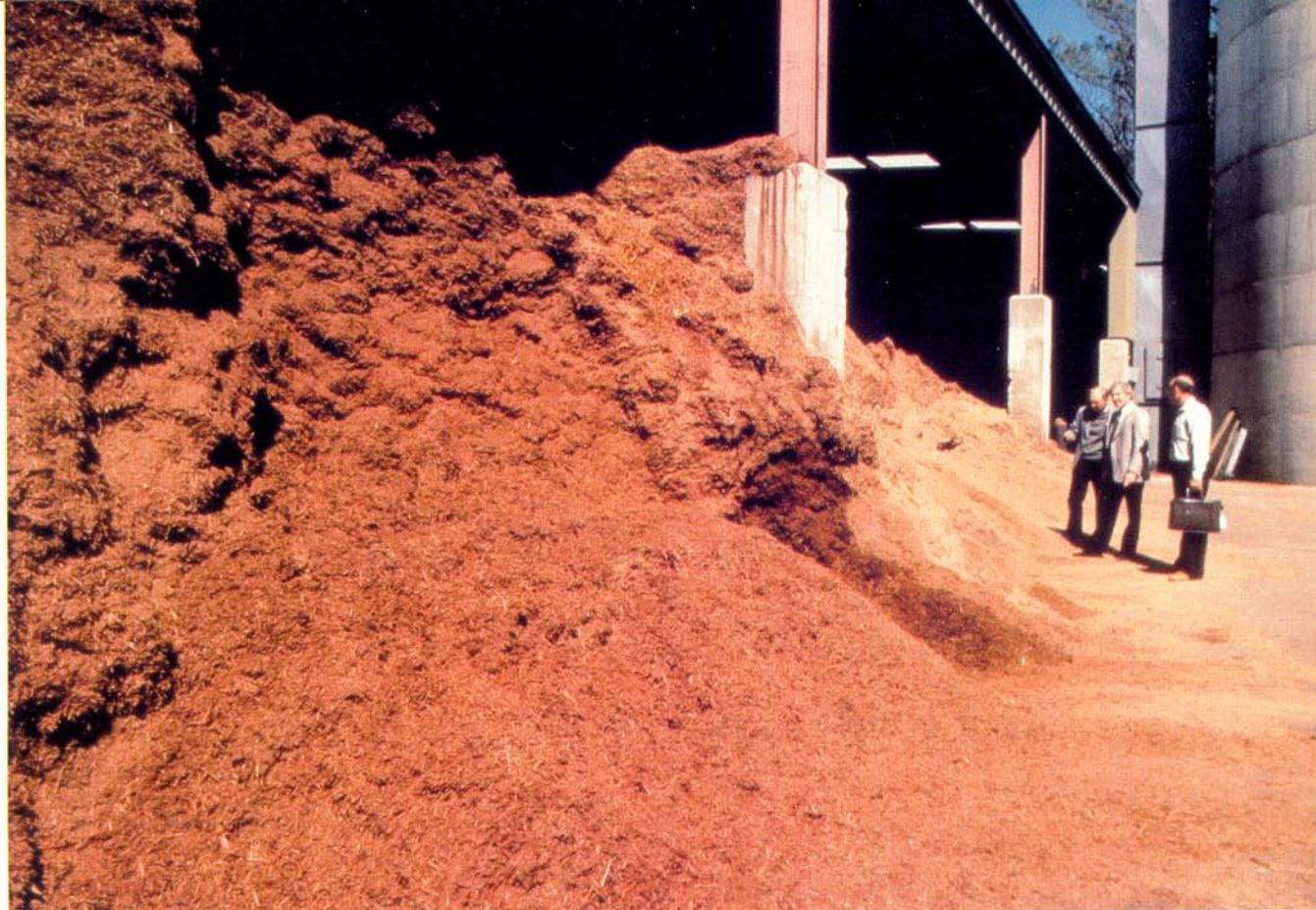
RESERVE WASTE STOCKPILE —Waste wood fuel users need to maintain reserve stockpiles as a hedge against supply disruptions. While most reserves are stored in covered buildings—such as above—bins and silos, open air storage is not rare.
